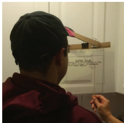
The augmented reality prototype was created by mounting transparencies with instructions on a hat.
